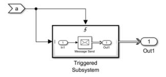
Here is an example of sending messages based on value changes (rising, falling, or either).
