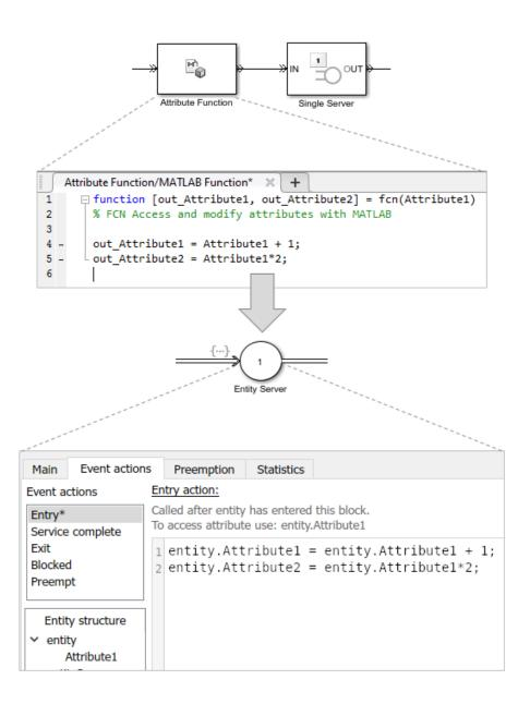
If you have longer or more complicated code, consider replacing the Attribute Function block with a Simulink Function and copying the code without modification into the Simulink Function block.
