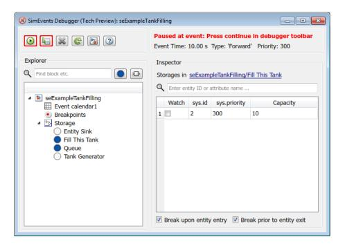
The simulation stops at the entity you opted to watch. As you continue the simulation or step through the model, the debugger stops at the various breakpoints and watchpoints that you set, letting you explore the model simulation.
