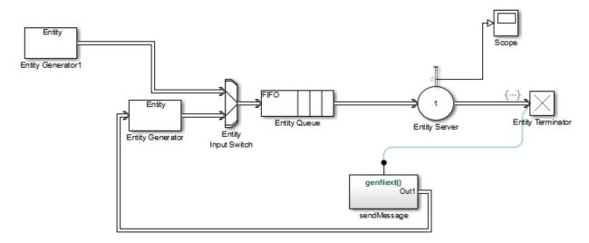
In this example, Entity Generator1 generates the first entity. SendMessage contains the genNext function, which sends a message.
