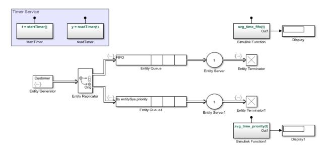
This example has four Simulink Function blocks. Two define timer functions, startTimer and readTimer. The other functions calculate average times.
