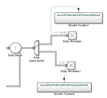
When preemption occurs, causing the Entity Server block to complete immediately service of all low priority tasks, one of the two Simulink Function blocks calculates the elapsed time of each departing task using the recordPreferredWaitTimes and recordNonPreferredWaitTimes functions. The two Entity Terminator blocks calls these Simulink Function to calculate the elapsed times.
