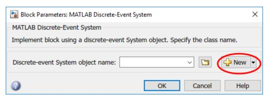
3 If the System object exists, enter its name in the **Discrete-event System object** name. Click the list arrow. If valid System objects exist in the current folder, the names appear in the list.
