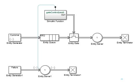
**Note:** A gate prevents new entities from arriving at the server but does not prevent the current entity from completing its service. If you want to eject the current entity from the server upon a failure occurrence, then you can use the preemption feature of the server to replace the current entity with a high-priority "placeholder" entity.
