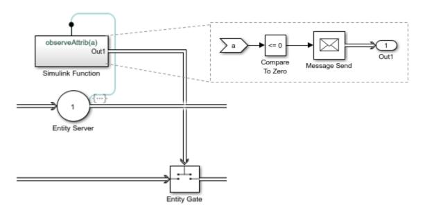
Here is an example of sending messages on trigger edges (rising, falling, or either).
