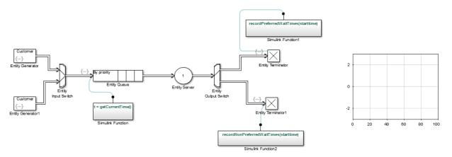
You can see from the plots that despite the shorter service time, the average system time for the nonpreferred customers is much longer than the average system time for the preferred customers.
