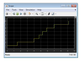
Upon generating each entity, the Entity Generator block reads the value of the input signal and uses that value as the time interval until the next entity generation.
