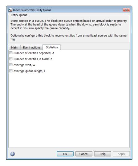
This procedure shows you how to access a statistical output signal for a given SimEvents block.
