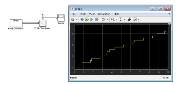
To generate entities with exponential random arrival times, in the **Intergeneration time action** field, enter MATLAB code that uses the **mean** function, for example:
