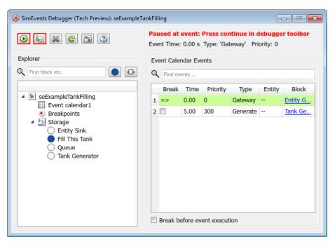
2 To inspect the attributes of an entity, click the **Fill This Tank** storage element in the **Explorer** pane.
