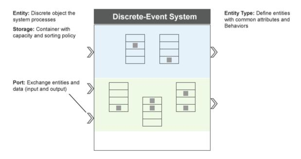
Ports enable a discrete-event system to exchange entities and data with other blocks or systems. A MATLAB discrete-event system supports a variable number of input and output ports using the <code>getNumInputsImpl</code> and <code>getNumOutputsImpl</code> methods. You can also specify which ports are entity ports and the entity types for these ports. Use the <code>getEntityPortsImpl</code> method to specify these port properties.
