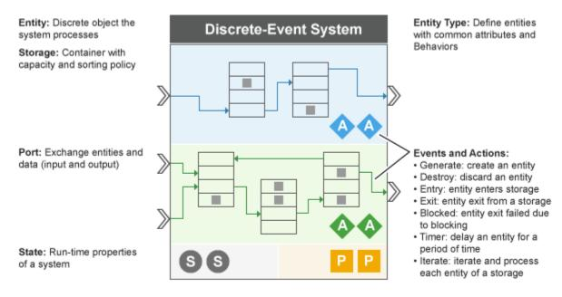
Parameters: Configurations of a system (Some are run-time tiunable)
