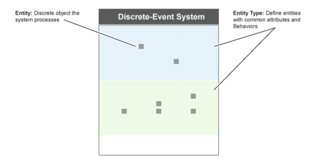
In a discrete-event system, an entity is a discrete object that the system processes. An entity has a type. An entity type defines a class of entities that share a common set of data specifications and run-time methods. Examples of data specifications include dimensions, data type, and complexity.
